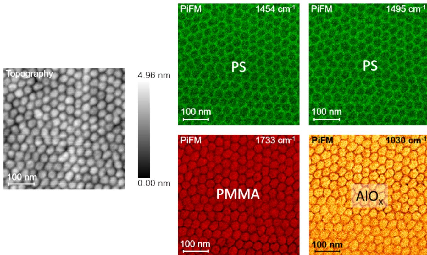
FIGURE 4: PiFM images and topography of hexagonal pattern of cylinder-forming PS-b-PMMA BCP after SIS processing.
