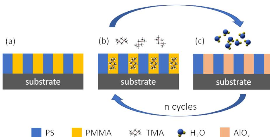
**FIGURE 1:** SIS of  $\text{AlO}_x$  in PS-b-PMMA BCP. (a) Prior to SIS processing; (b) During interaction with TMA vapor when TMA infiltrates PMMA selectively; (c) Exposure to water vapor converts TMA to aluminum oxide. Cycle is repeated  $n$  times.
