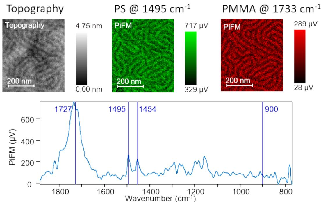
FIGURE 2: PiFM spectrum and images of PS and PMMA blocks in PS-b-PMMA BCP prior to SIS processing; note the equal block width of PS and PMMA molecules.
