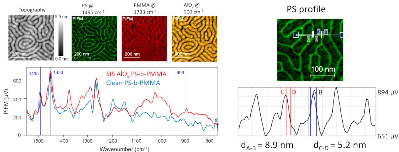
FIGURE 3: PiFM spectrum and images of PS-b-PMMA after the SIS processing. The region bounded by the white dotted square in the PS map is magnified for defining the PS cross-section profile; the PS width has shrunk to ~9 nm in width.
